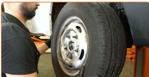
Utskifting: stabilisator foring – FORD Transit Mk5 Minibuss (V184, V185).
