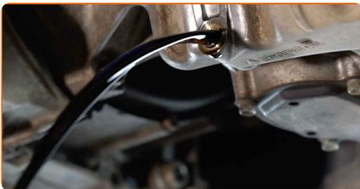
Utskifting: motorolje og oljefilter – HONDA Accord I Hatchback (SJ, SY). Tips:
