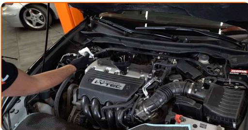
Utskifting: motorolje og oljefilter – HONDA Accord I Hatchback (SJ, SY).
