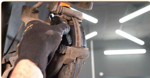
**Utskifting: bremseklosser – INFINITI Q70 (Y51). Tips:**
