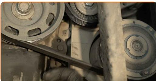
Utskiifting: vannpumpe + registerreimsett – SKODA Fabia II Hatchback (542).
