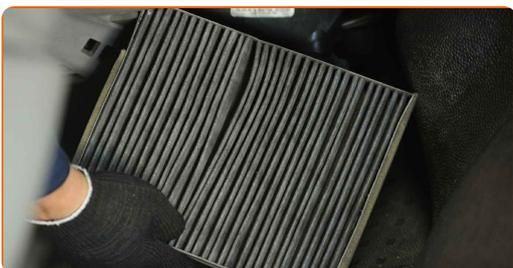
Utskifting: kupefilter – VW California T6 Minibuss (SGC, SGG, SHC). Tips:
