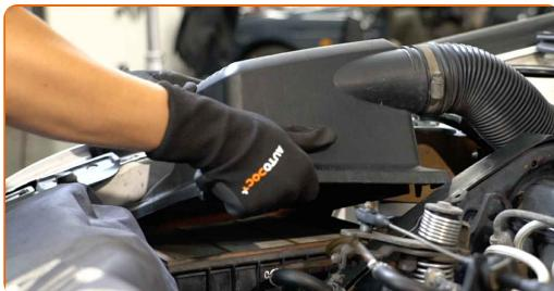
**5** Fjern filterelementet fra filterhuset.
