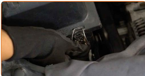
**4** Løft opp dekselet til luftfilterhuset litt.
