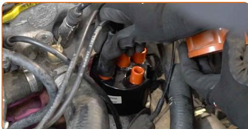
**Utskifting: fordelerotor – VW Passat B2 Hatchback (32B). AUTODOC
