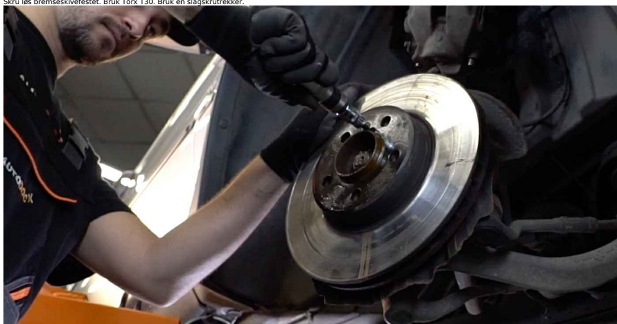
Utskifting: bremsekiver - BMW X5 E53. Tips:
